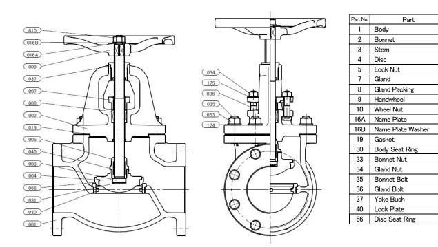
This illustration shows typical construction. Refer to the approved drawing for disassembly and assembly.
