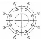
1.3.8 Increase line temperature and pressure gradually at test operation. Retighten the threaded areas, if needed.
